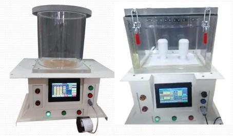
The ASTM D5094 Vacuum Leak Test for Bottles, Containers, and Caps is a standard procedure for testing leaks in non-carbonated beverages and similar liquids, ensuring compliance with international standards. Burhani Engineering Technology manufactures this Bottle Leak Test Chamber for detecting leaks based on the ASTM D5094 method, commonly used in the beverage industry.
